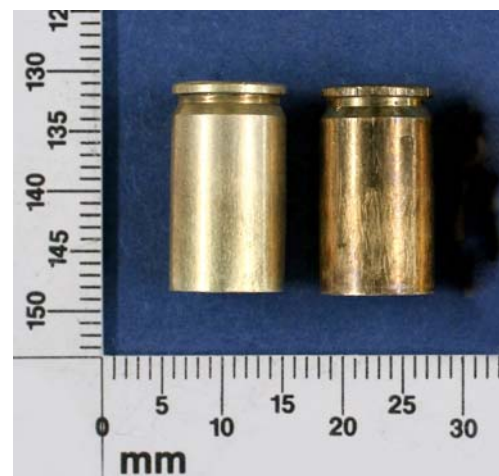
Fig. 2 The effect of lysis buffer on casings. Left a casing treated with lysis buffer. Right a casing that was untreated. Both casings came from the same batch
